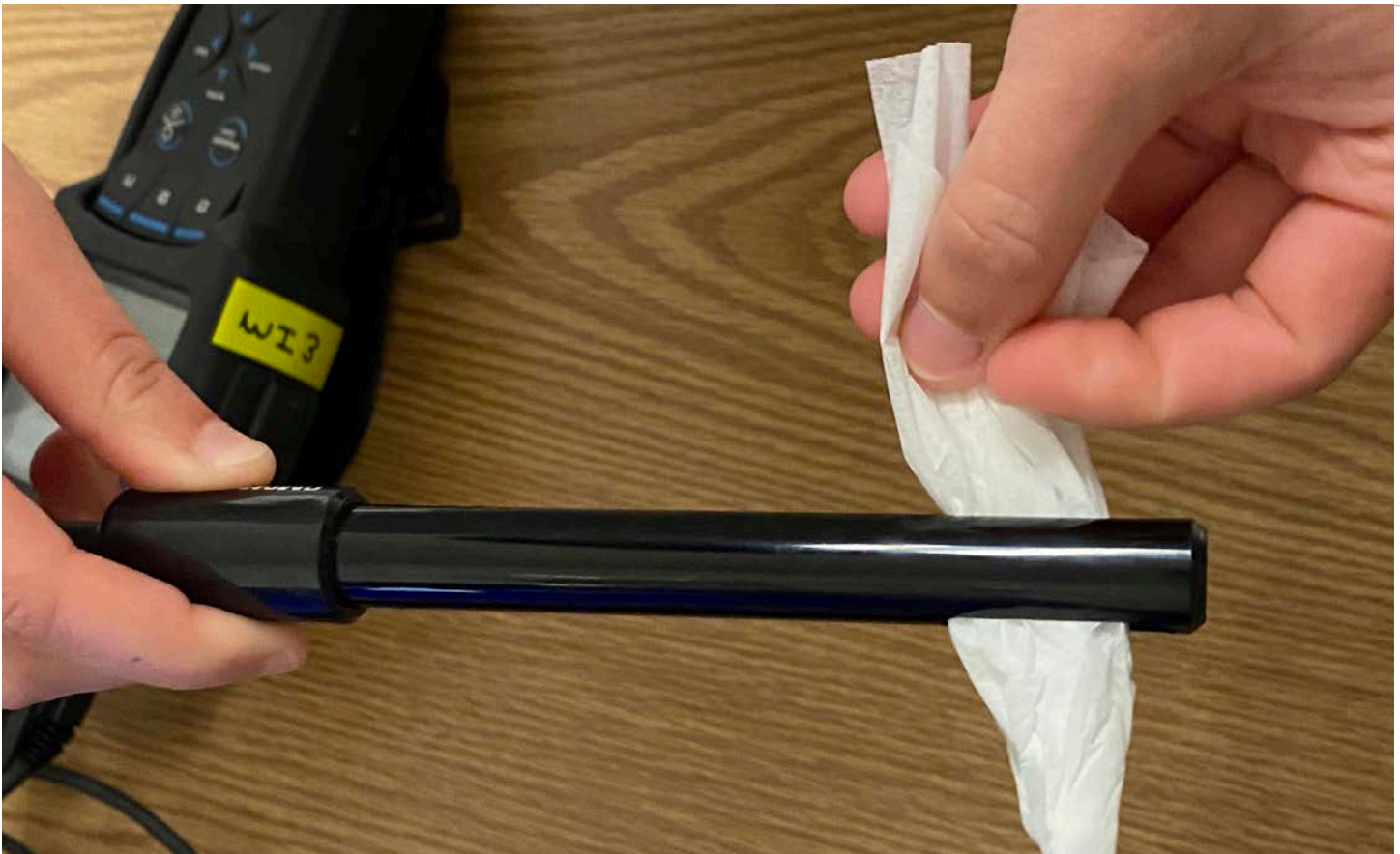
Figure 11: It is important to dry the interior portion of the conductivity probe.
