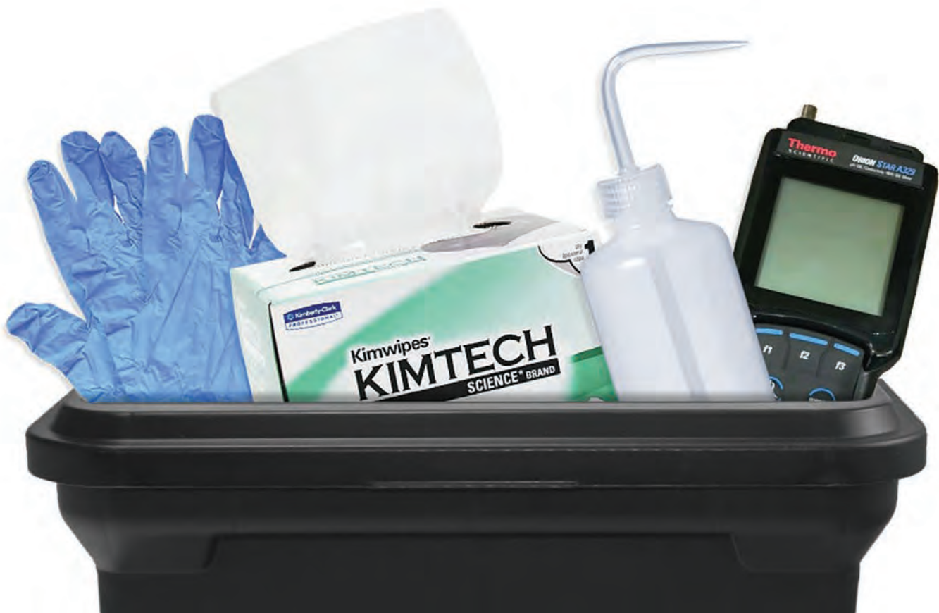
Figure 4: Field bin with gloves, Kimwipes, DI water squirt bottle, and Orion Star A329 meter.
